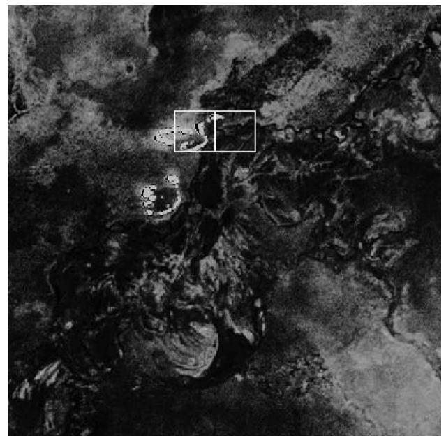
Fig. 7. Example of 1 km-MOD14 fire pixels (white squares) over corresponding ASTER scene. Bright ASTER pixels are saturated pixels in the 2.43- \mu m channel and correspond to the flaming front of the fire. Also evident is an undetected fire to the lower left of the detected fire.
